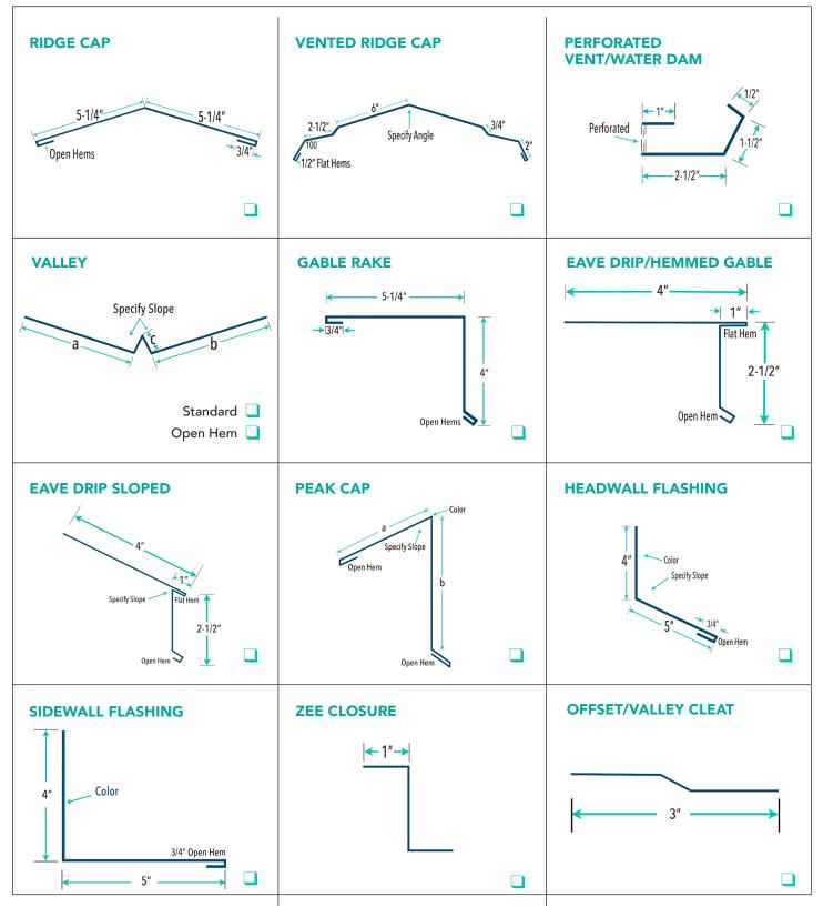
Custom flashings and trim available upon request. Contact EMF for additional information. The items listed are for a typical installation. Installers should determine products required for a specific project based on applicable regulations, product approvals, building codes, and accepted industry practices.
