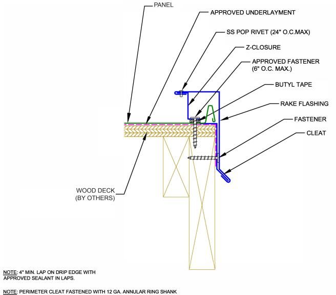
NOTE: PERIMETER CLEAT FASTENED WITH 12 GA. ANNULAR RING SHANK NAIL OR #10 DIAMETER SCREW, 10" O.C.AT PERIMETER ROOF AREAS AND 6" O.C. AT CORNER ROOF AREAS.
