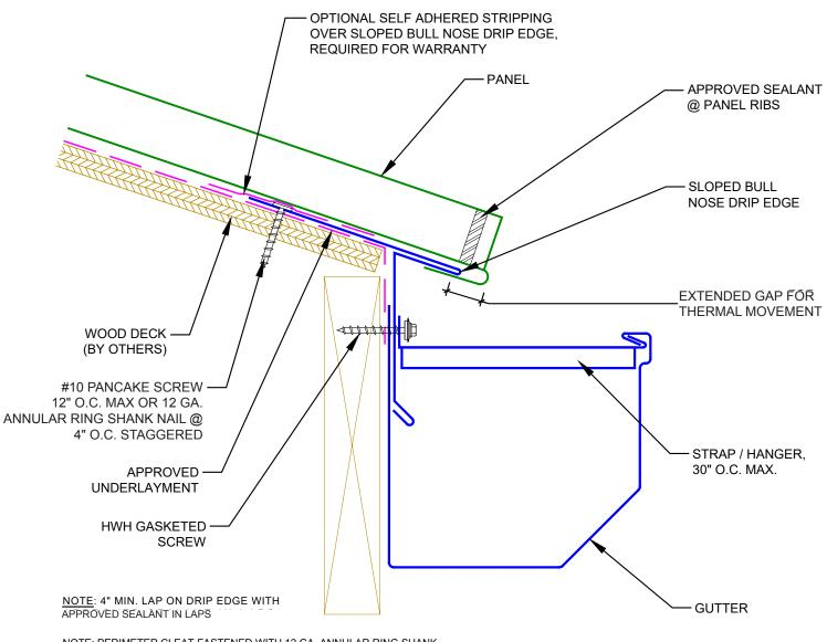
NOTE: PERIMETER CLEAT FASTENED WITH 12 GA. ANNULAR RING SHANK NAIL OR #10 DIAMETER SCREW, 10" O.C.AT PERIMETER ROOF AREAS AND 6" O.C. AT CORNER ROOF AREAS.
