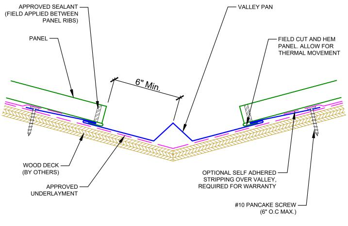
NOTE: FLASHING LAPS IN VALLEY ARE 6" MIN. USE TWO ROWS OF APPROVED TUBE SEALANT IN ALL LAPS.
