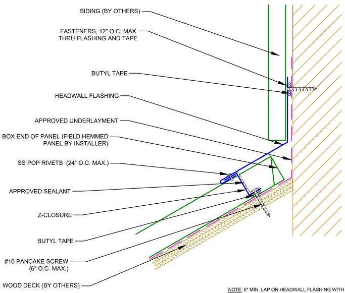
NOTE: 6" MIN. LAP ON HEADWALL FLASHING WITH APPROVED SEALANT IN LAPS.
