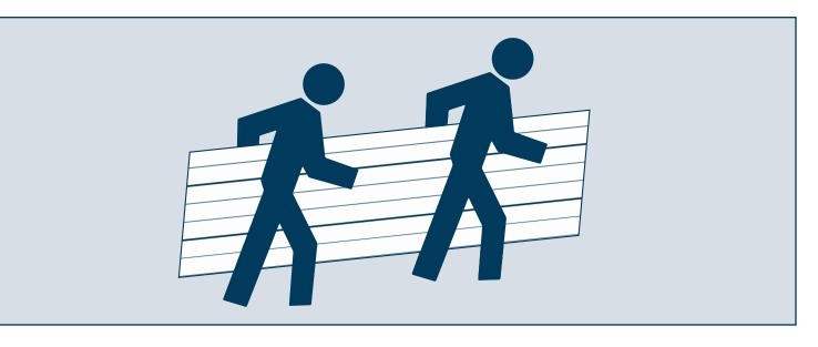
**Once a bundle is opened, individual panels must be handled with care to prevent panel buckling or finish damage.** Never slide a panel over another panel when removing it from the bundle. A panel should be lifted up from the bundle in order to minimize the possibility of damaging the finish.
