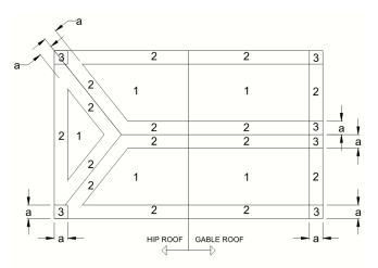
a: 10% OF LEAST HOIZONTAL DIMENSION OR 0.4h, WHICHEVER IS SMALLER, BUT NO LESS THAN EITHER 4% OF LEAST HORIZONTAL DIMENSION OR 3FT (0.9M). OR AS DETERMINED BY DESIGN OR OTHER APPLICABLE CODE.
