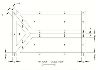
8: 10% OF LEAST HOLZON I AL DIMENSION OR 0.4h, WHICHEVER IS SMALLER, BUT NO! LESS THAN EITHER 4% OF LEAST HORIZONTAL DIMENSION OR 3FT (0.9M). OR AS DETERMINED BY DESIGN OR OTHER APPLICABLE CODE.
